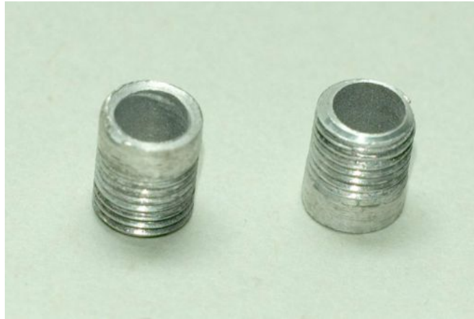
Fig. 4: Cementing caps from aluminum.
